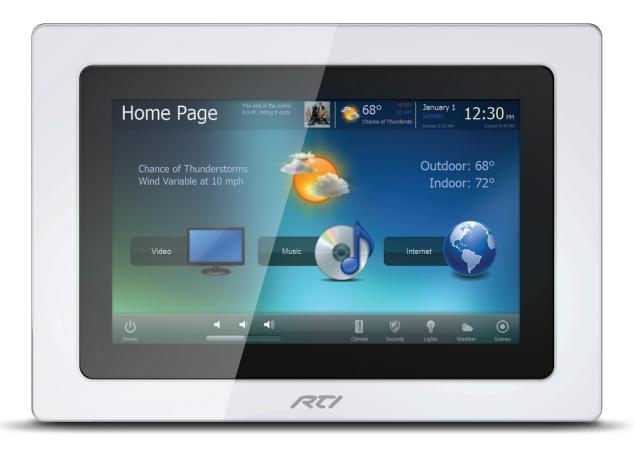
The KX7 is designed for sophisticated installations that require a touchpanel with the size and power to take command of a room's environmental and media technology. With advanced features like a multi-touch capacitive touchscreen, direct IR/RS-232\* control and analog video inputs, the KX7 possesses the style and user-friendliness required to fit any type of setting.
