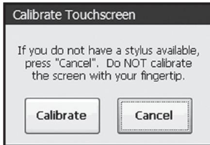
Follow the directions on the display to complete the calibration process.
